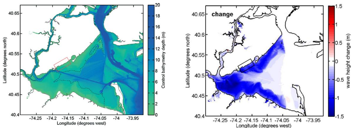
The models showed that oyster reefs significantly reduced wave height and wave energy for both storms. Wave height reduction was very sensitive to reef height, but not to reef roughness. Peak average flood level was only changed by a very small amount by the presence of reefs, and the direction of change varied by storm. Together, the sediment analysis and modeling indicate that large, well-established oyster reefs can provide protection for storms by decreasing the height and
