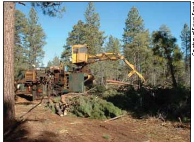
Figure 3-7—Chain flail debarker feeds chipper on White Mountain Stewardship Contract.
