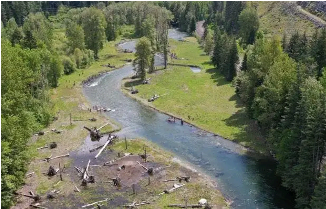
Aerial view of the site two years after construction, showing the remeandered channel and floodplain on the left and the filled-in former channel on the right.
