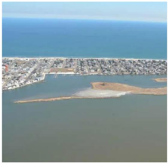
Upon completion of placement of dredged material, the north end is now reconnected to the main portion of the island, contributing significantly to coastal resiliency.
