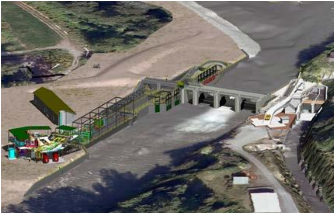
Complete CAD design of the new barrier structure and fish passage facility.
