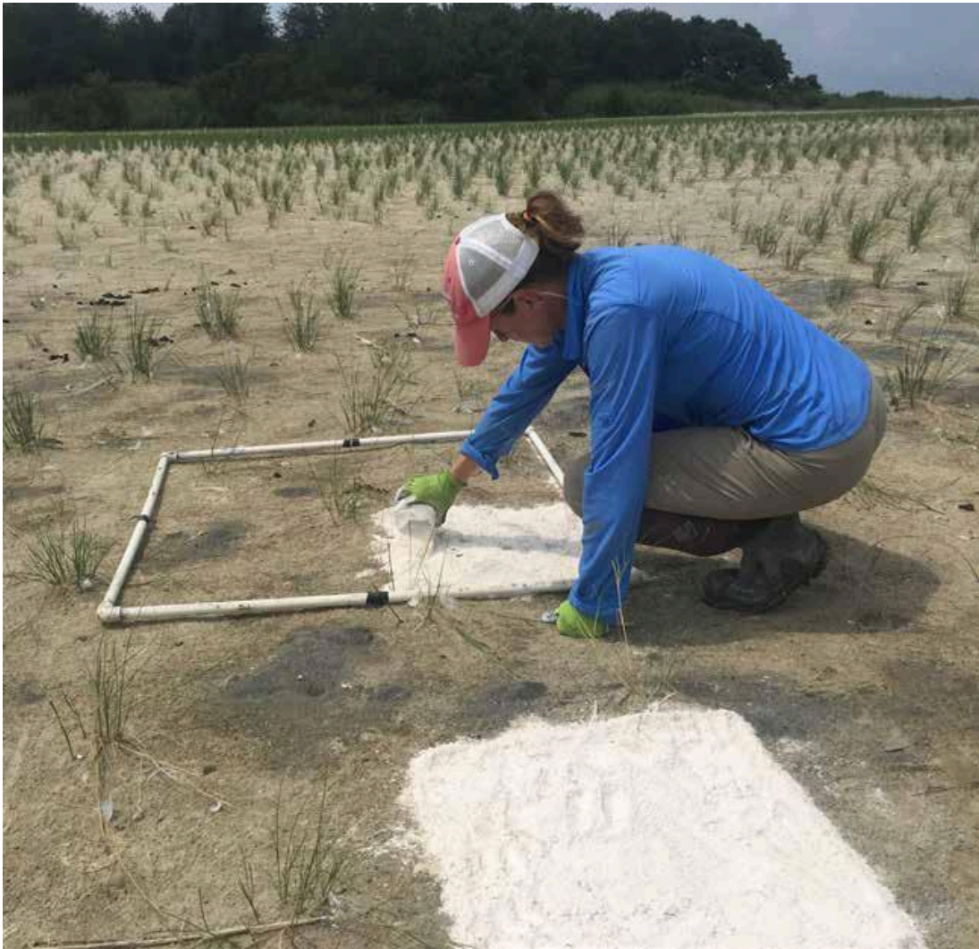
Placing feldspar clay on sediment to determine the amount of sediment accretion. (Photo by NOAA)
