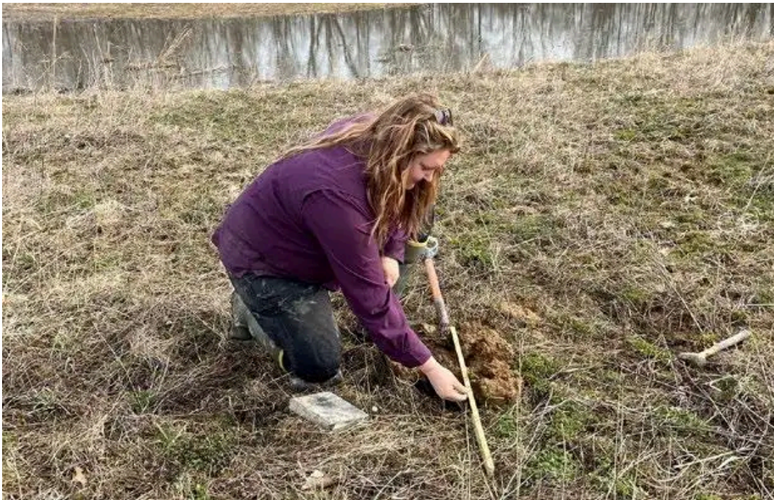
A soil scientist collects samples and completes a soil description in Cell 4. Measurements were used to monitor hydric soil conditions and nutrient retention through time.
