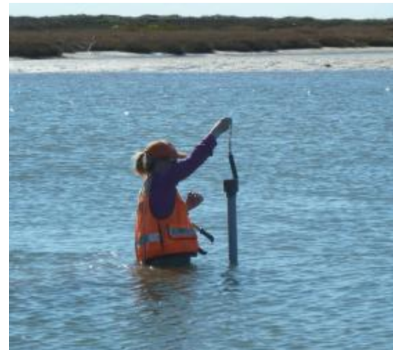
A USGS technician deploys a water logger at Seal Beach National Wildlife Refuge. Data from loggers provide detailed information on flooding and drainage patterns in the marsh, including depth during tidal cycles, inundation periods for the salt marsh plain, and characteristics of flooding during storm events.
